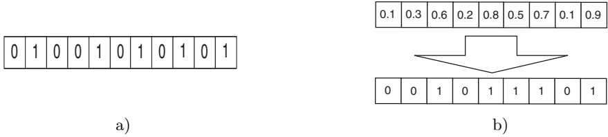
Fig. 2. Solution encoding using: a) binary encoding, b) real encoding
